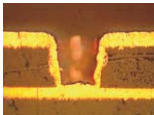
Microvia d=75 µm, 18 µm Cu, 63 µm 1080
